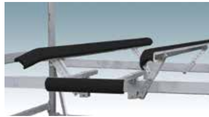
Pivoting Bunks — Carpeted wood or aluminum and vinyl bunks conform to and cradle the boat's hull; double set of bunks is required for 8,000 lbs and 10,000 lbs lifts.
